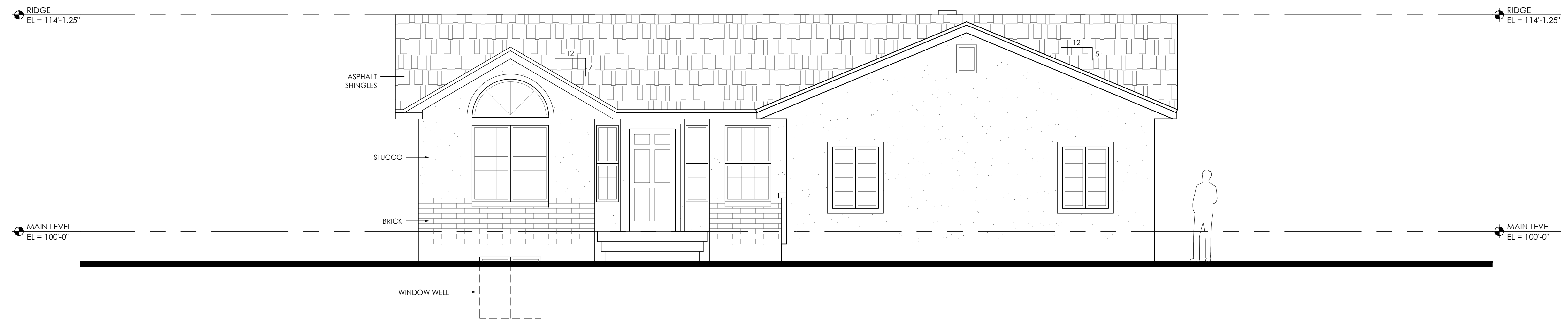
PROPOSED A SOUTH ELEVATION SCALE: 1/4" = 1'-0" 0 1 2 4 8
